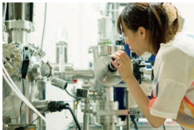
Material properties studied by x-ray photoelectron spectroscopy Analysis of electronic Structures and properties of air-sensitive matters using x-ray photoelectron spectrometer
