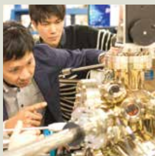
Measurement of the electronic state by photoelectron spectroscopy
